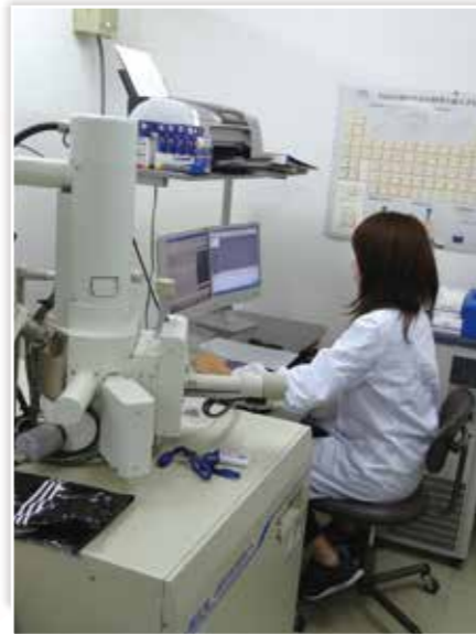
■ Scanning electron microscope Performs fine structure observation of sample surface. ■ Energy dispersive X-ray analyzer Performs qualitative and quantitative analyses of elements in the sample.
