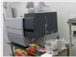
■ Inductively coupled plasma emission spectroscopy Analyzes trace elements of ppb order.
