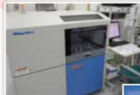
■ X-ray fluorescence analyzer Analyzes elements in sample qualitatively and quantitatively using X-rays.
