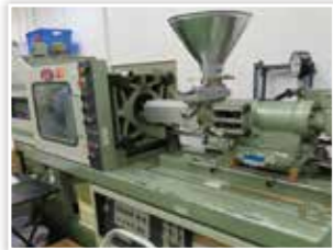
■ Injection molding machine Creates sample products through injection of molten material into a mold to produce test specimens for assessing workability and performance of polymer additives.
