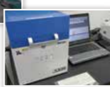
■ X-ray fluorescence analyzer Analyzes elements in sample qualitatively and quantitatively using X-rays.
