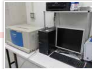
■ Particle size analyzer Analyzes particle size and particle size distribution in powder.
