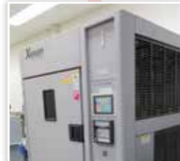
■ Weathering test instrument Evaluates weather resistance of test specimens in a short duration by means of accelerated weathering.
